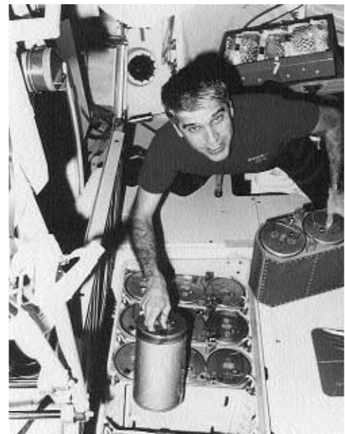
Sidney Gutierrez changes the filters of the air supply system on board the Space Shuttle. The system doesn't actually recycle air but conserves resources by filtering the air.
