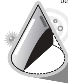
4. Hyperbola- section cut at an angle greater than the angle of the slope of the cone.
